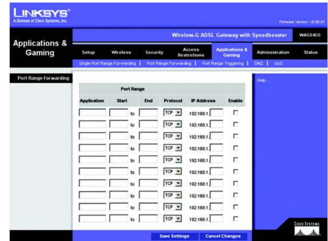
Figure 6-30 : Port Range Forwarding (Transfert de connexions)
